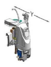
• YAxis: The depth wise stroke is operated by a single central brushless motor with adjustable speed (0-20 mt/min) and overload switch limit. Motion is obtained on linear guideways with revolving balls pads protected by bellows. Maximum sturdiness and accuracy are ensured by inclined teeth rack and pinion transmission with patented lose correction system.
