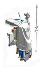
• **Z Axis:** The verticle motion of the operating head is effected on linear guideways with revolving balls pads protected by bellows with adjustable speed 0-12 m/min.
